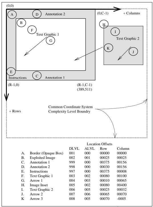
FIGURE 8. NITF Display Level (DLVL) illustration.
